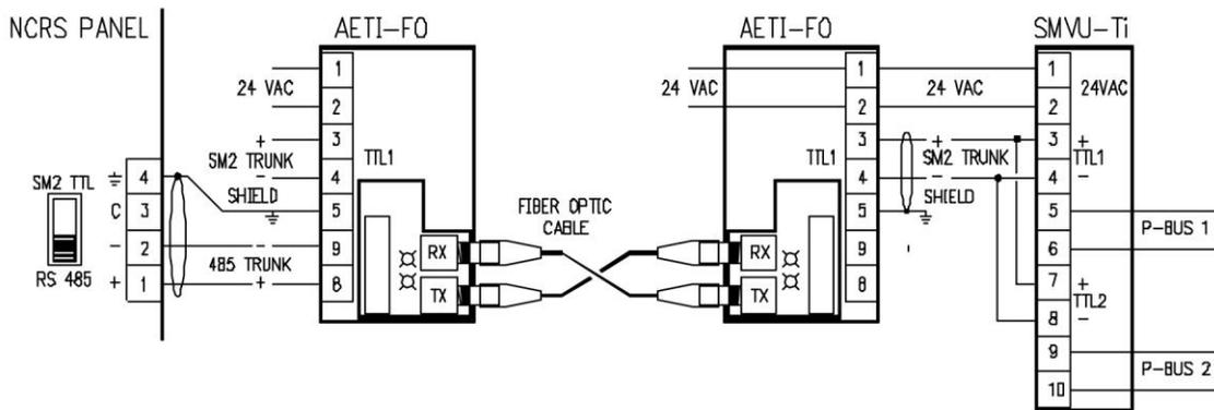
This application depicts the use of the AETI-FO transducers and a SMVU-Ti P-Bus interface. The AETI-FO transducers will repeat the 2400 baud TTL or RS-485 signals from the NCRS panel and interface to STAEFA's SMVU-Ti1P-bus interface. By connecting the AETI-FO's SM2 TTL I/O port up to both the SM2 TTL ports on the Ti you are able to run two P-bus trunks of 50 + SMVU controllers.
